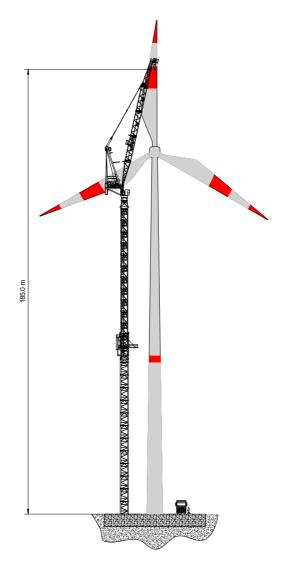
Our latest wind turbine adapted luffing jib cranes provide exceptional performance and are optimised to suit the build and maintenance of wind farms.
